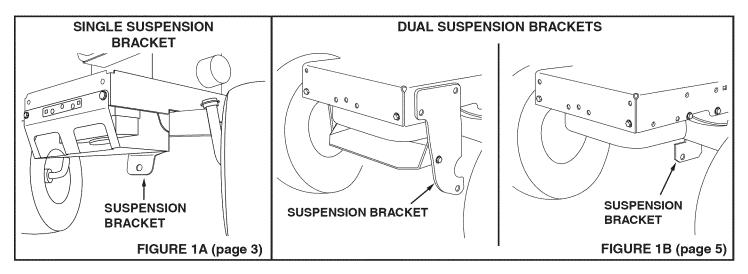
For all tractors with model numbers beginning with 917, look under the front of your tractor (Figure 1A & 1B). If there is a single mower deck suspension bracket located underneath the middle of the front axle, continue on to INSTRUCTIONS FOR SINGLE SUSPENSION BRACKET TRACTORS on page 3. If your tractor does not have a mower deck suspension bracket underneath the middle of the front axle, skip to INSTRUCTIONS FOR DUAL SUSPENSION BRACKET TRACTORS on page 5.
